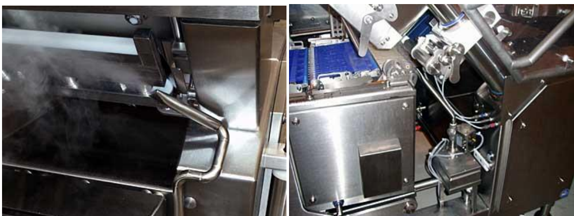
Figure 3. Germ Nebulization module at the slicer knife and at conveyor belts (air-solution.com)
