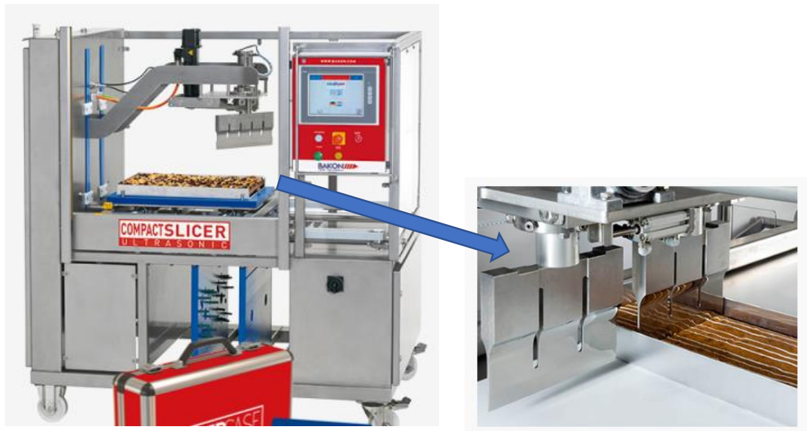
Figure 1. Ultrasonic cutting machine for bakery (Source. https://bakon.com/ )
